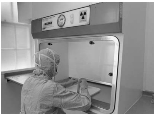
Figure 7.1. Example of a radiopharmaceutical laminar flow safety cabinet, MAT-I-MAT.
